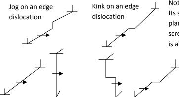
Note the jog is also an edge dislocation. Its slip plane is perpendicular to the glide plane of parent dislocation. The kink is a screw dislocation. Its direction of motion is along the length of the dislocation.
